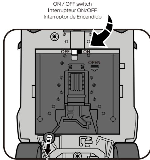
• Remove screw to lift cover. Slide battery door to flip open.
